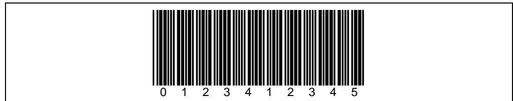
Fig. 6-1: Bar code pattern (Code 39; module width 0.35 mm (11.8 mil); Print ratio 2:1)
